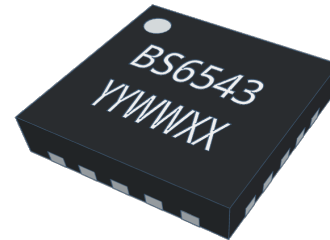
3mm x 3mm x 0.55mm, 20-Lead QFN Package
