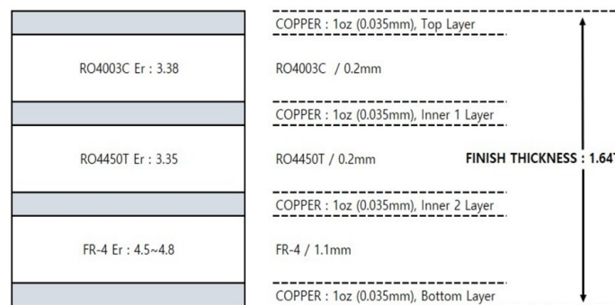
Figure 27. Evaluation Board PCB Layer Information
